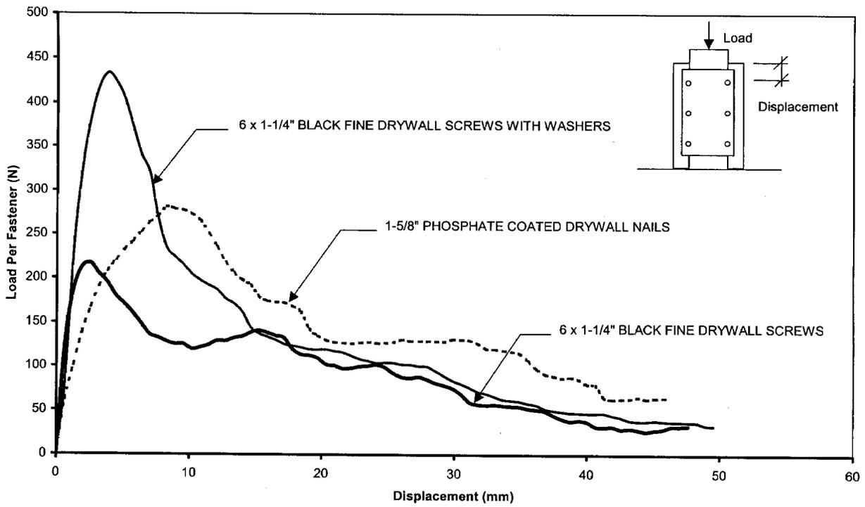
Figure 4. Comparison of Force-Displacement for Gypsum Wallboard Fasteners.
