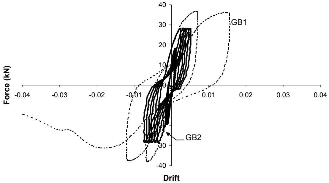
Figure 3. Lateral Force vs. Wall Drift for 2440x2440 Gypsum Wallboard Shear Walls.
