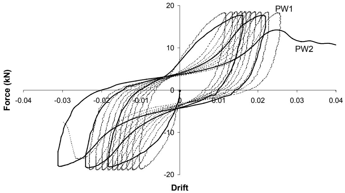
Figure 1. Lateral Force vs. Wall Drift for 2440x2440 Plywood Shear Walls.
