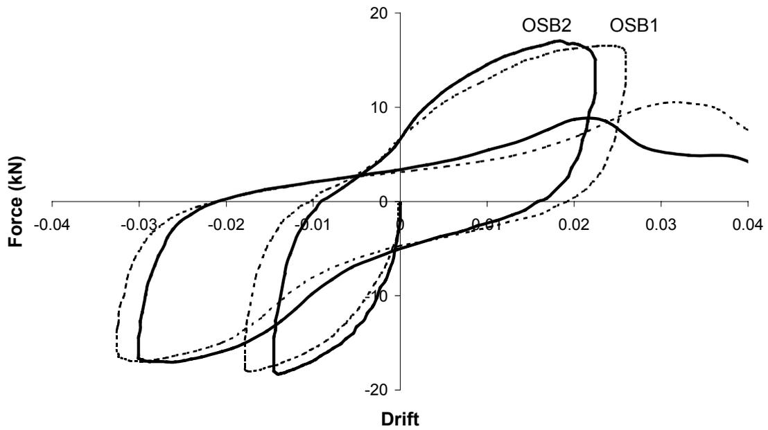
Figure 2. Lateral Force vs. Wall Drift for 2440x2440 Oriented Strand Board Shear Walls.
